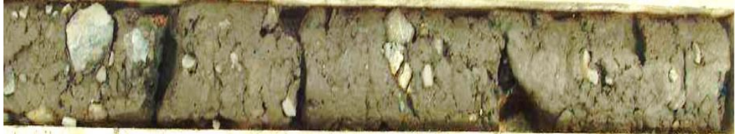
Figure 5.6: Example of 'Dublin' Boulder Clay
